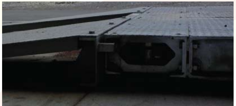
END LOADCELL AND RAMP
