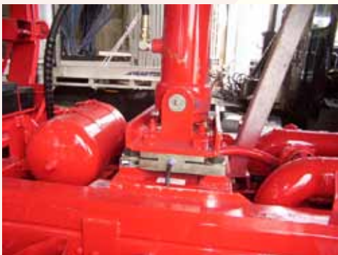
RAM LOADCELL INSTALLATION
